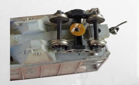
Un-peel the protective paper from the tag and place the tag on the Car/Locomotive over the trucks screw cylinder or the lowest point of the car/engine body.
